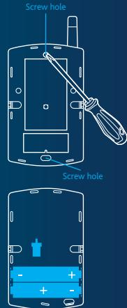
**NOTE:** The control panel will be required to be in test mode before you can change the batteries on the sensor.
