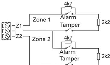
Figure 7. Connecting Fully-Supervised Loop (FSL) zones
