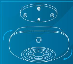
Avoid mounting it in direct sunlight or any objects blocking the lens, so the detection is not affected.
