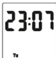
**Note:** During time/date setting, when the Adv/Ovr or Boost buttons are held down, the setting under adjustment will advance or decrease more rapidly
